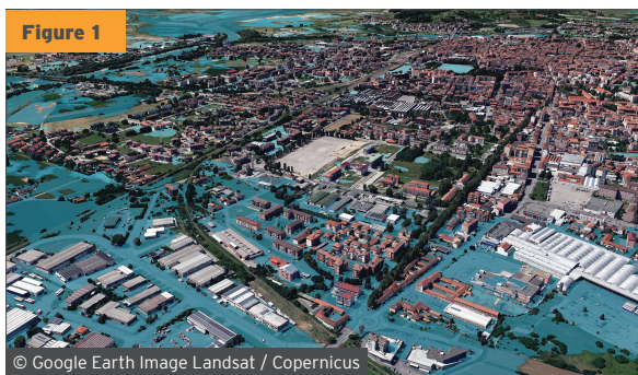
Figure 1 River and Surface Water flood extent for the 100-year return period, Asti.
