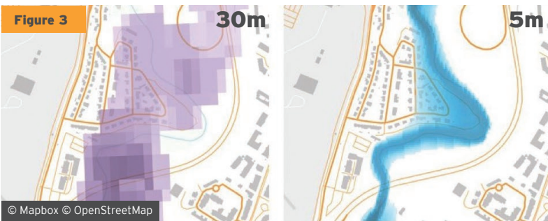
Figure 3 Effect of the map resolution on risk assessment. At 5m resolution, JBA's flood maps provide clearer definition of the river channel and floodplain compared to coarser resolution mapping.
